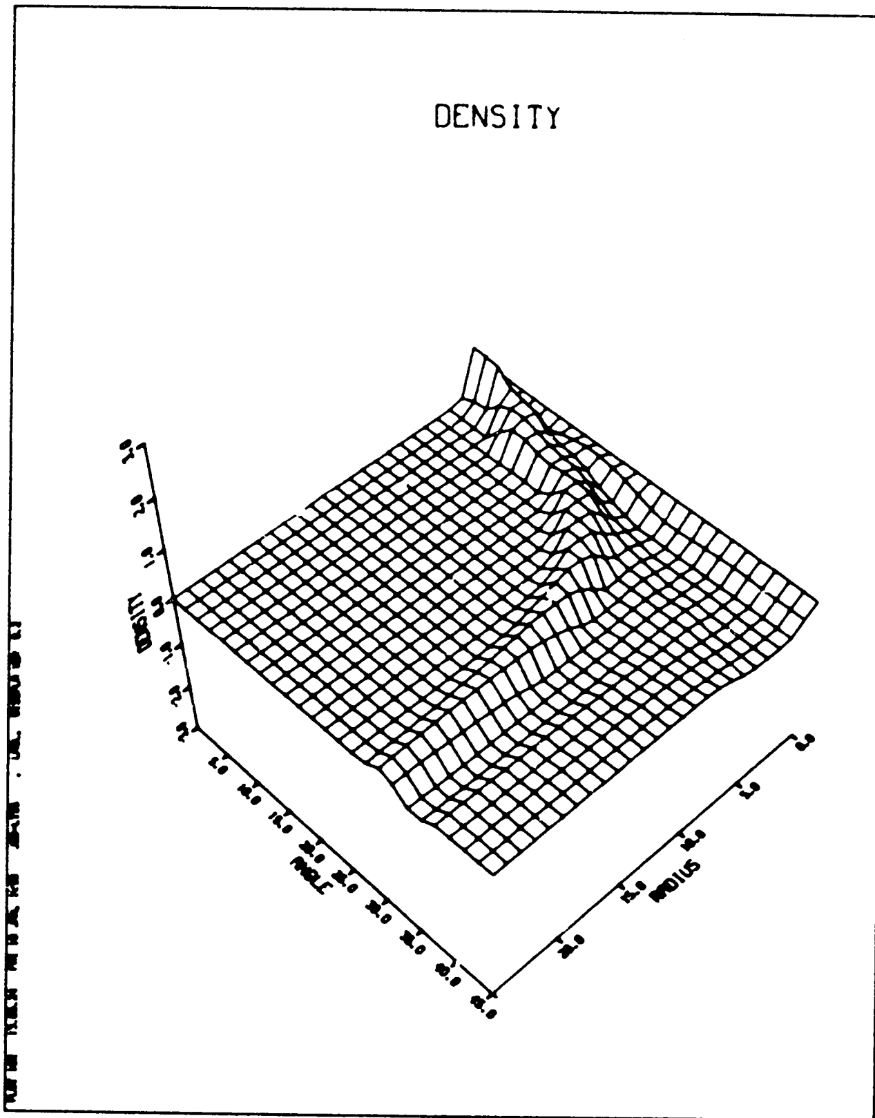
Fig. 9. Shock wave just reaching the axis of rotational symmetry near the origin of coordinates. Note the structure of the axially directed shock.
